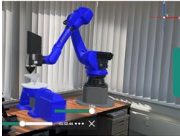
Figure 7: Simulation with AR applying SKM DCAM. This can be forwarded to all partners and seen locally. The screenshot displays the process working on top of a real office desk.
