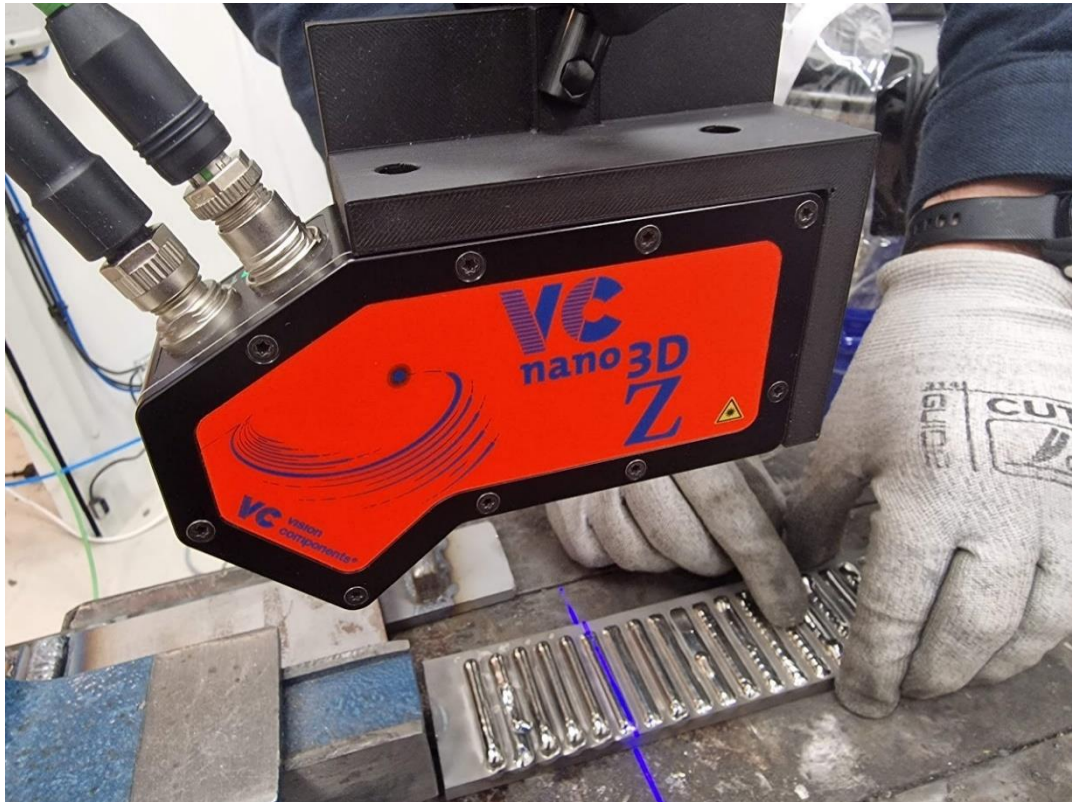
Figure 9: In the picture, a small version of the VC nano 3D Z that is used to evaluate depositions from the ALABAMA project. Mounting the scanner to a robot, SINTEF has made a software to extract and utilise the scan data.
