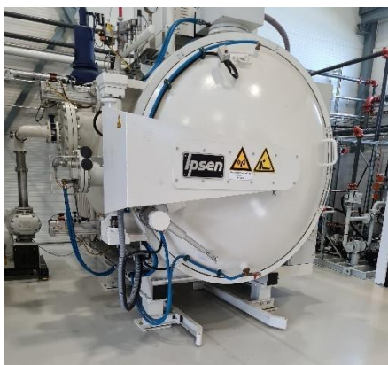
Figure 23: Ipsen Heat Treatment Furnace
